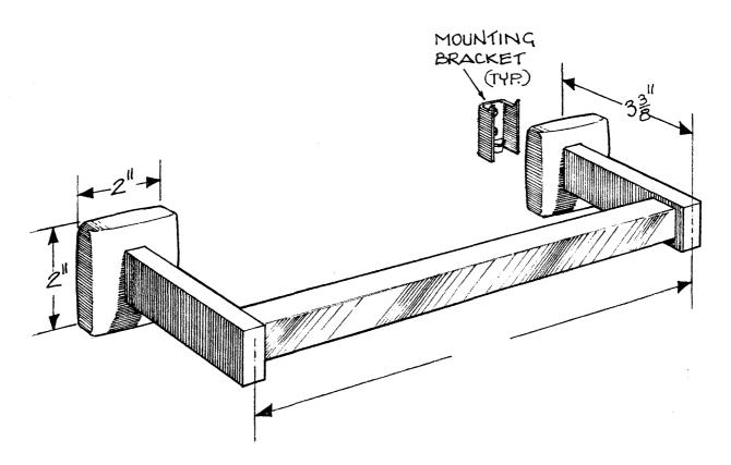
**CONSTRUCTION:** END BRACKETS are type 304 brite stainless steel.
