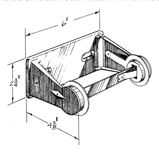
CONSTRUCTION: Fabricated of chrome plated heavy gauge steel with riveted
