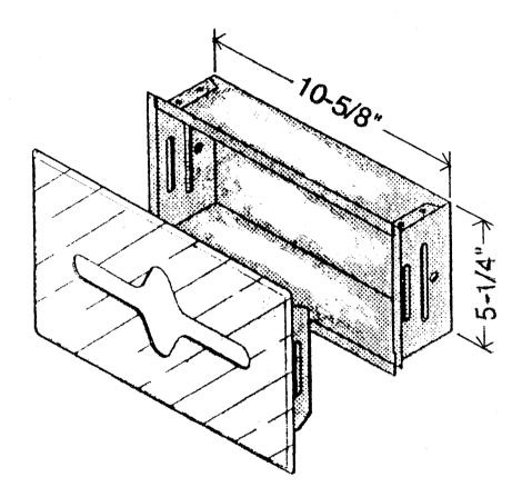
CONSTRUCTION: FACEPLATE FABRICATED OF CHROME PLATED STEEL.
