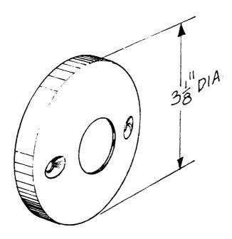
CONSTRUCTION: 1"(104A) or 1 1/4"(105A) hole size x 3 1/8" diameter #304 satin stainless
